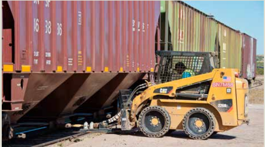
This custom hopper gate opener attachment was home-built by Apache Railway mechanical forces using Alco crank-shaft support bearings and other components they had on hand.
