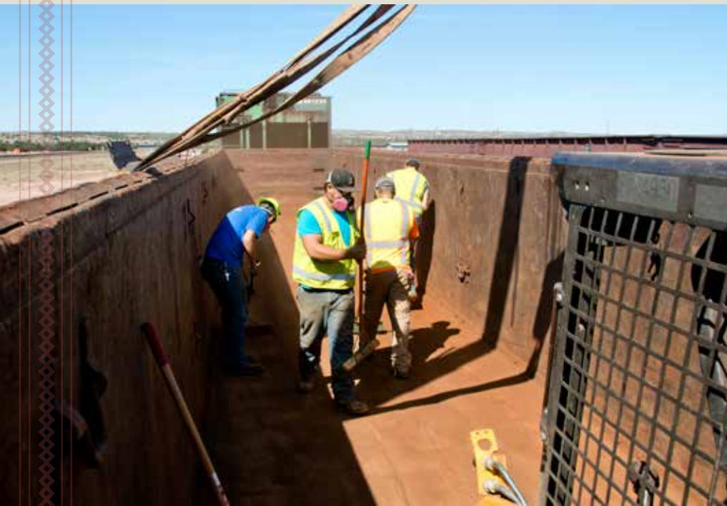
Dry car cleaning can be hot and dusty work. A team of workers use push brooms to complete the cleanout of a mill gondola.
