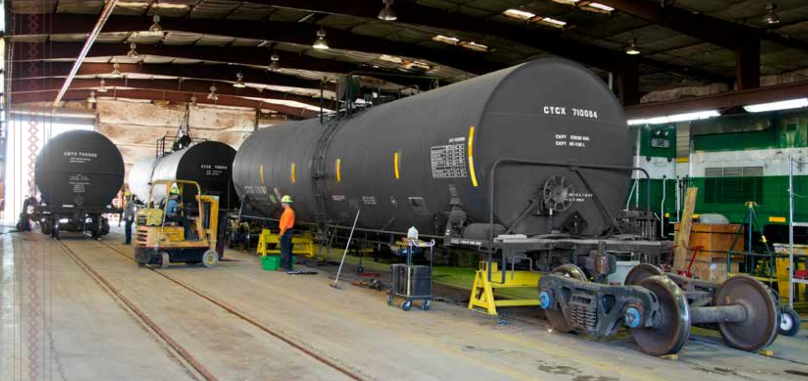
The Apache Railway is home to a four-track car and locomotive maintenance facility near Snowflake, Ariz. This shop is operated by the railway to primarily perform contract tank-car repair and qualification work.
